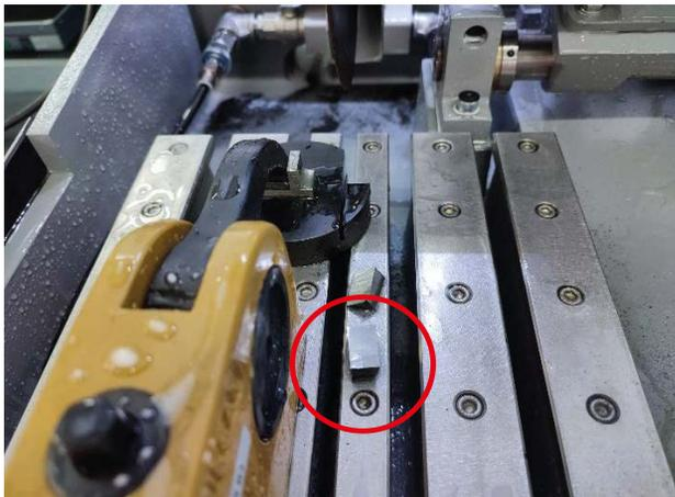
After cutting operation, samples mounted with Diallylphthalat (DAP) polymeric powder in ECOPRESS 102 press.
