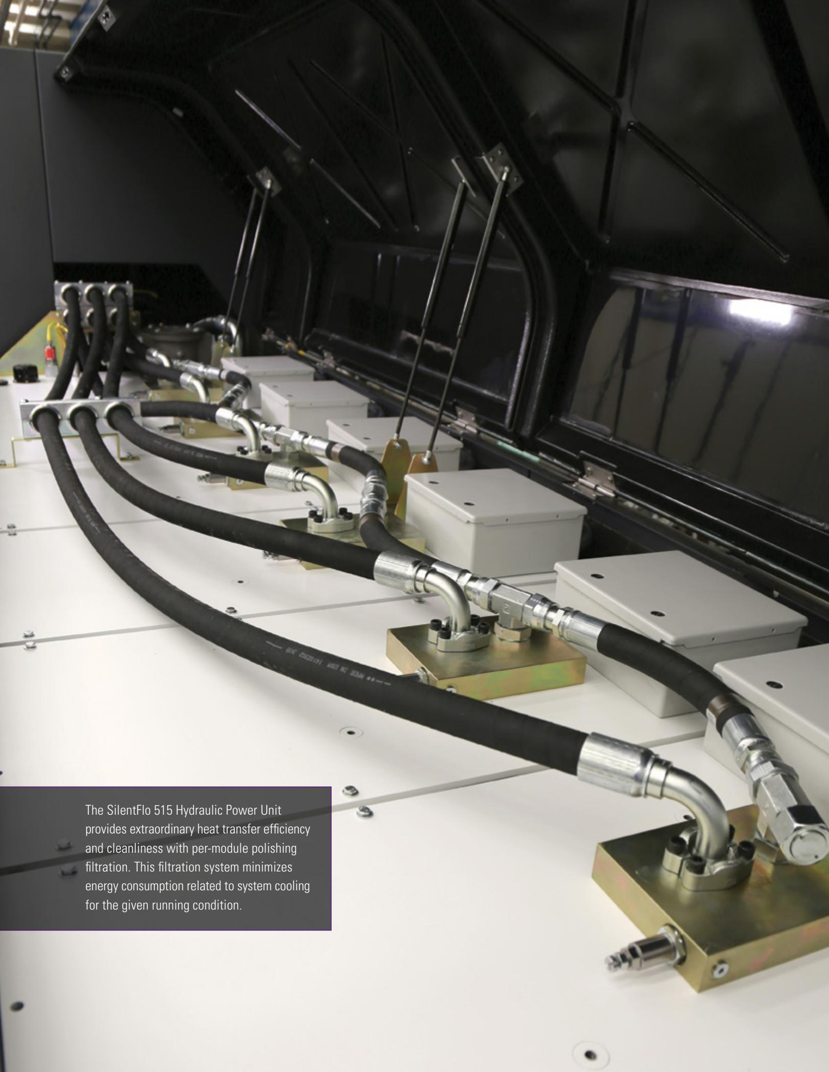
The SilentFlo 515 Hydraulic Power Unit provides extraordinary heat transfer efficiency and cleanliness with per-module polishing filtration. This filtration system minimizes energy consumption related to system cooling for the given running condition.
