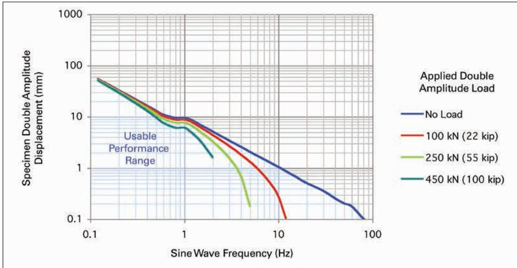
ACTUATOR STATIC FORCE: 500 kN (110 kip)      LOAD FRAME MODEL: 370.50
