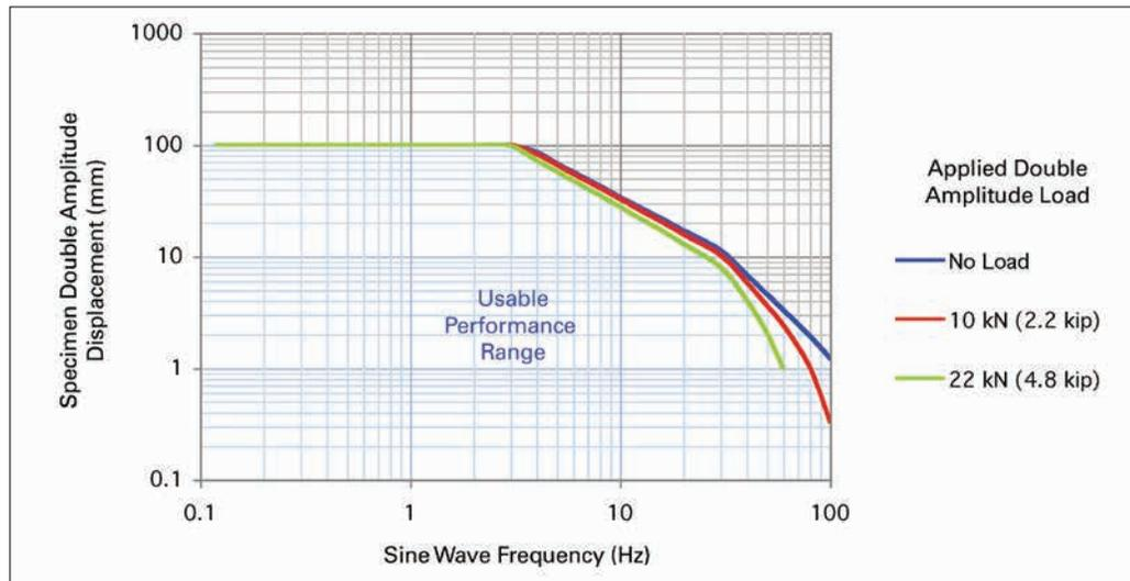
ACTUATOR STATIC FORCE: 25 kN (5.5 kip)
