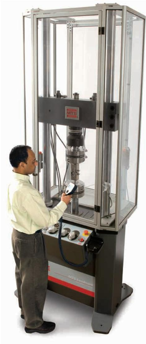
an ergonomic body position. The compact system handset provides the ultimate in test setup convenience, featuring a clear test status display, precision controls for fine actuator positioning and an ergonomic design for both right- and left-handed operators.
