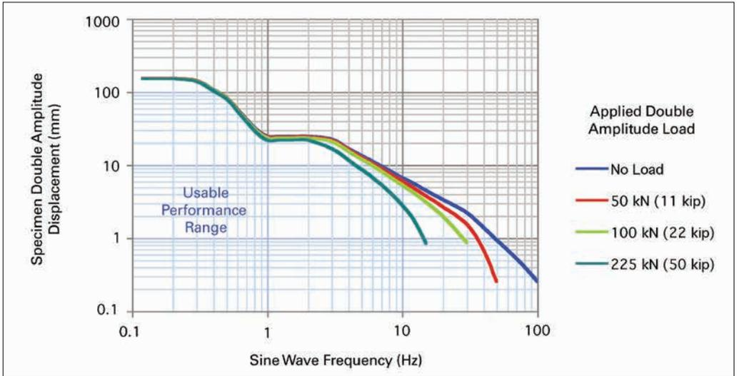
ACTUATOR STATIC FORCE: 250 kN (55 kip)
