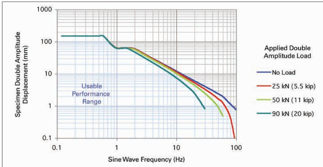
ACTUATOR STATIC FORCE: 100 kN (22 kip)      LOAD FRAME MODEL: 370.10
