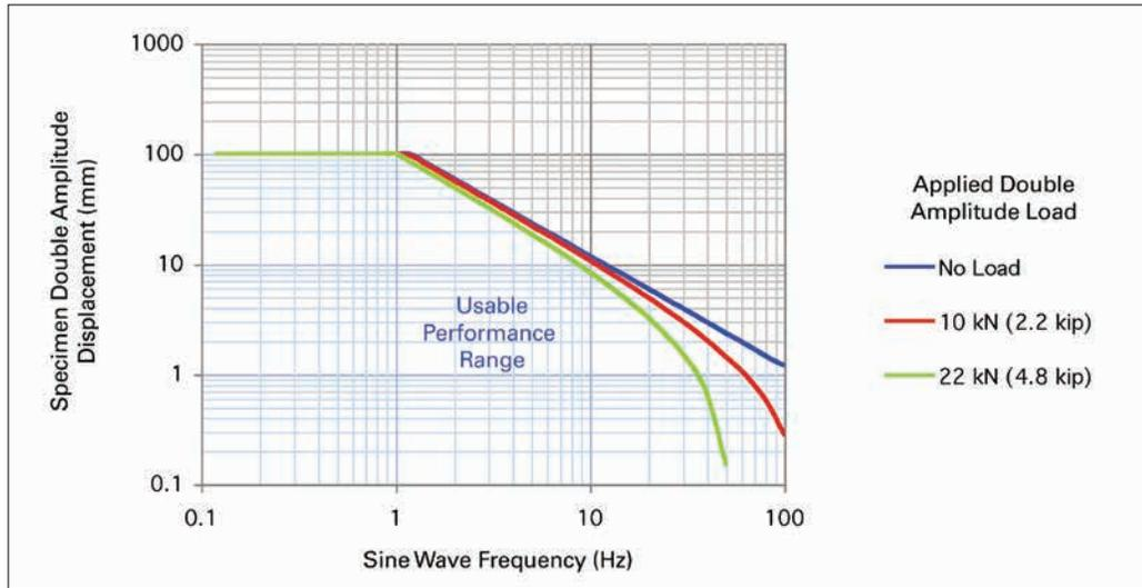
ACTUATOR STATIC FORCE: 25 kN (5.5 kip)
