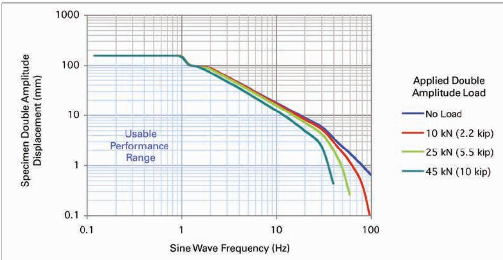
ACTUATOR STATIC FORCE: 50 kN (11 kip)
