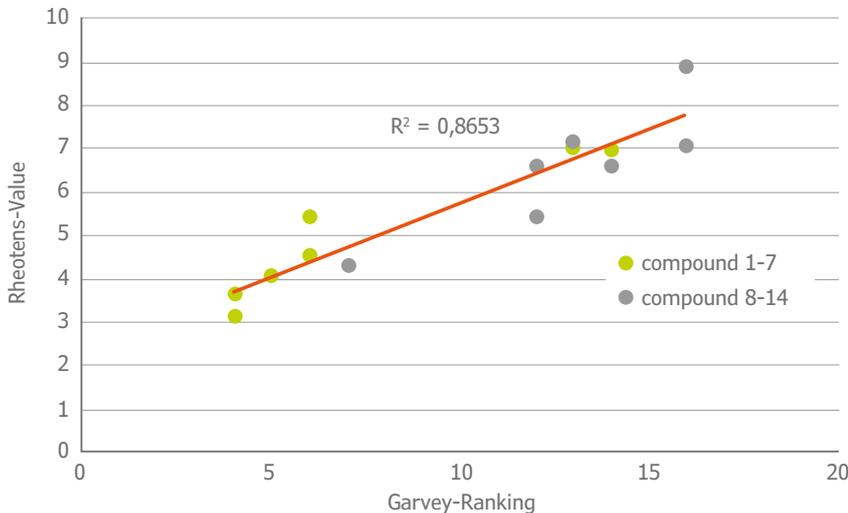
For elastomers, this results in a good correlation to the extrudate quality manually evaluated using the complex extrusion test with the Gravey die, which is also more prone to errors due to this manual evaluation.
