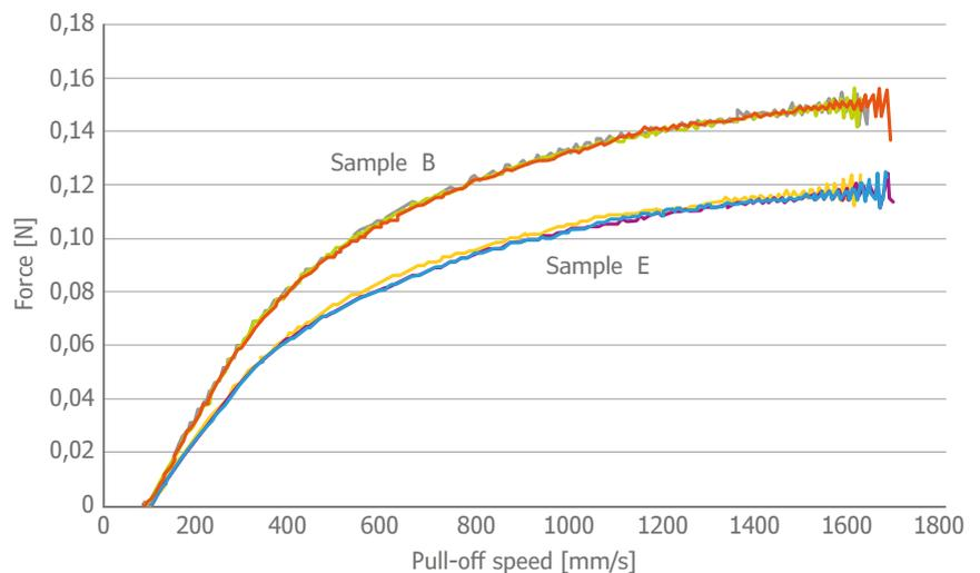
According to the manufacturer, sample B indicates a somewhat broader molecular mass distribution ( $M_w/M_n=11.1$ ) than sample E ( $M_w/M_n=10$ ). The RHEOTENS curves, each reproduced three times, indicate a clear increase in the melt strength of sample B compared to sample E.
