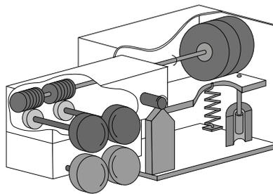
The functional diagram shows the RHEOTENS 71.97 with tandem pull-off wheels, which can also be retrofitted to older devices.
