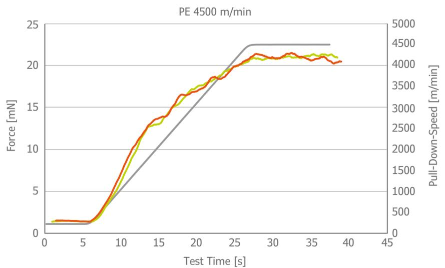
A typical test method is the ramp test up to the desired pull-off speed with a short speed holding phase. In the case of a mono filament, the material can also be wound up at the pull-off wheel without any appreciable increase in speed.
