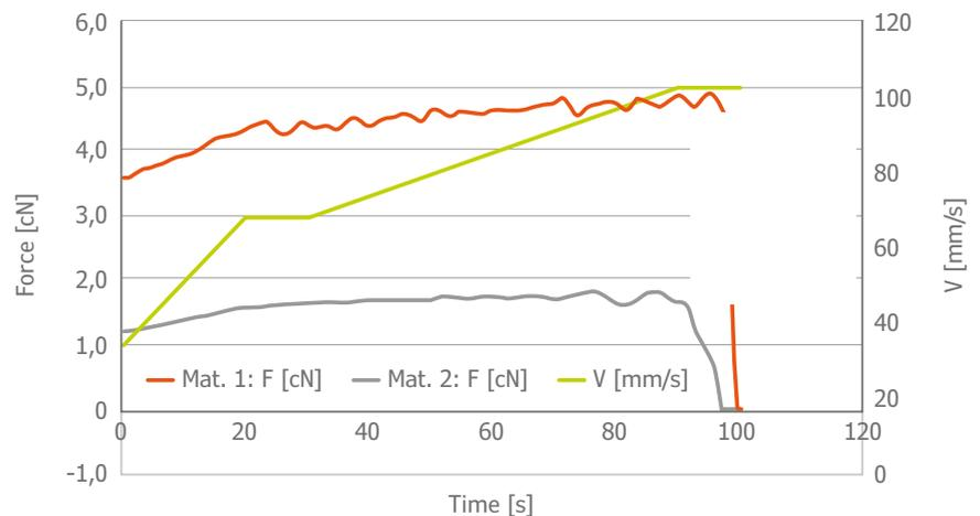
The following comparison shows the considerably higher selectivity of the test method compared to the pure melt index measurement. The simple operation, short measuring time and low speeds make this method particularly suitable for quality assurance during compound release or in incoming goods inspections.
