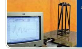
Economical uniaxial seismic simulator for basic research and
