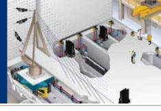
Affordable uniaxial controllers employ the same technology as the larger systems, but are efficiently packaged to control only a single actuator. Uniaxial controllers can be located near the seismic simulator and easily relocated with changing test setups.
