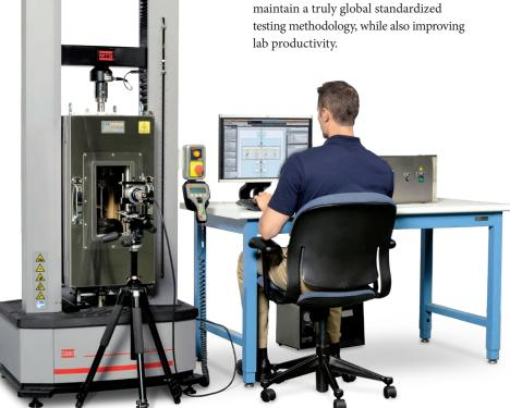
MTS TestSuite TW software applies drag-and-drop simplicity to allow for the monotonic or cyclic testing of textiles, plastics, metals, composites, adhesives, ceramics, foam and other materials, at both low- and high-force capacities.
