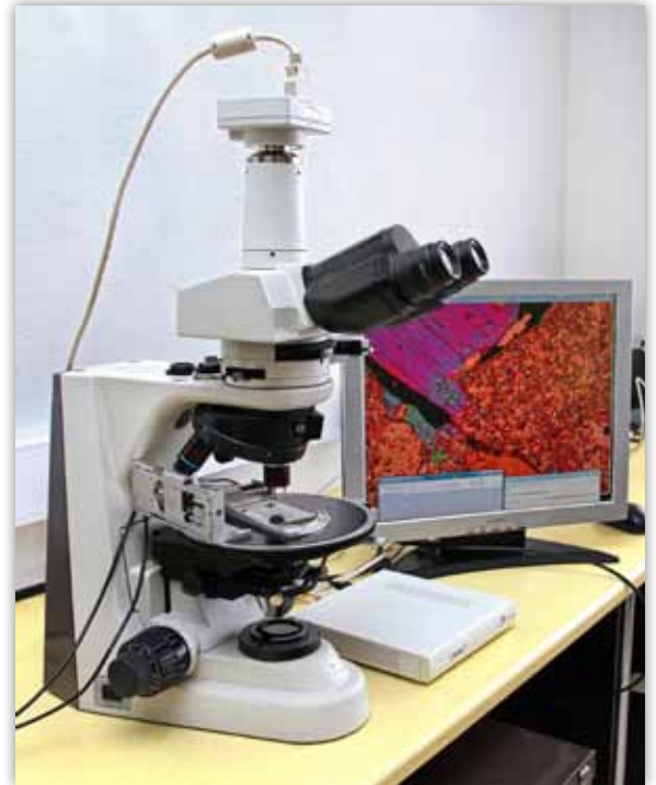
The PETROG system comprises a Nikon Eclipse 50iPOL binocular microscope fitted with a Nikon Digital Sight DS-Fi2 5-megapixel camera which relays overlapping photographs of the rock sample to a computer for analysis via a Nikon FireWire control unit, DS-U3.
