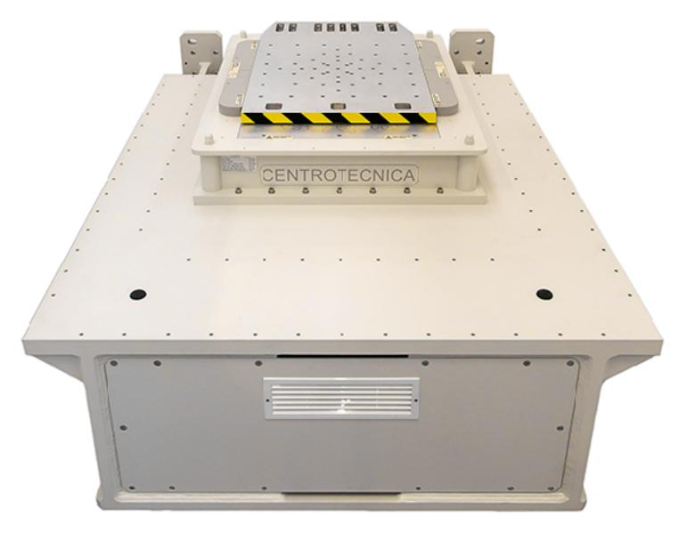
The slip tables are interchangeable with the same base. In this way the optimum solution for the most efficient energy consumption can always be achieved. The optional front cover ensures that circulating oil does not come into contact with the sample. In some areas (such as aerospace), safeguarding the cleanliness of the sample is essential.
