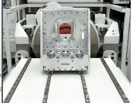
CENTROTECNICA has taken the concept of weight saving to the extreme by developing the RT fixture solution: fixtures that mount directly onto the RT slip table rails, eliminating the need for a table.
