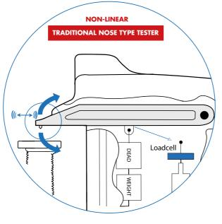
Traditional nose type hardness testers have the disadvantage that the indenter is fixed to a long load application arm that makes a circular movement. Due to this construction, the indenter is not only pushed but also dragged through the material with horizontal displacement.
