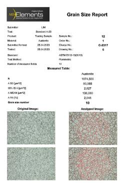
Complete measurement results in Report including the number of measured fields or images, the number of grains and the grain area (mean, minimum and maximum) using NIS-Elements
