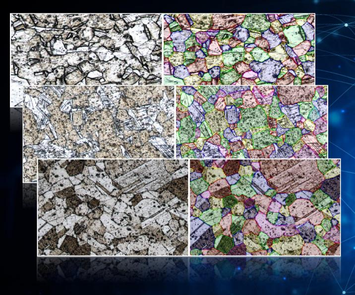
Reliable AI grain detection currently works primarily on Austenitic and Ferritic one-phase structures.
