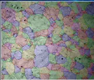
Al network is trained to correctly identify individual grains also on the images with shading. Achieving such excellent results is very difficult using common segmentation methods.
