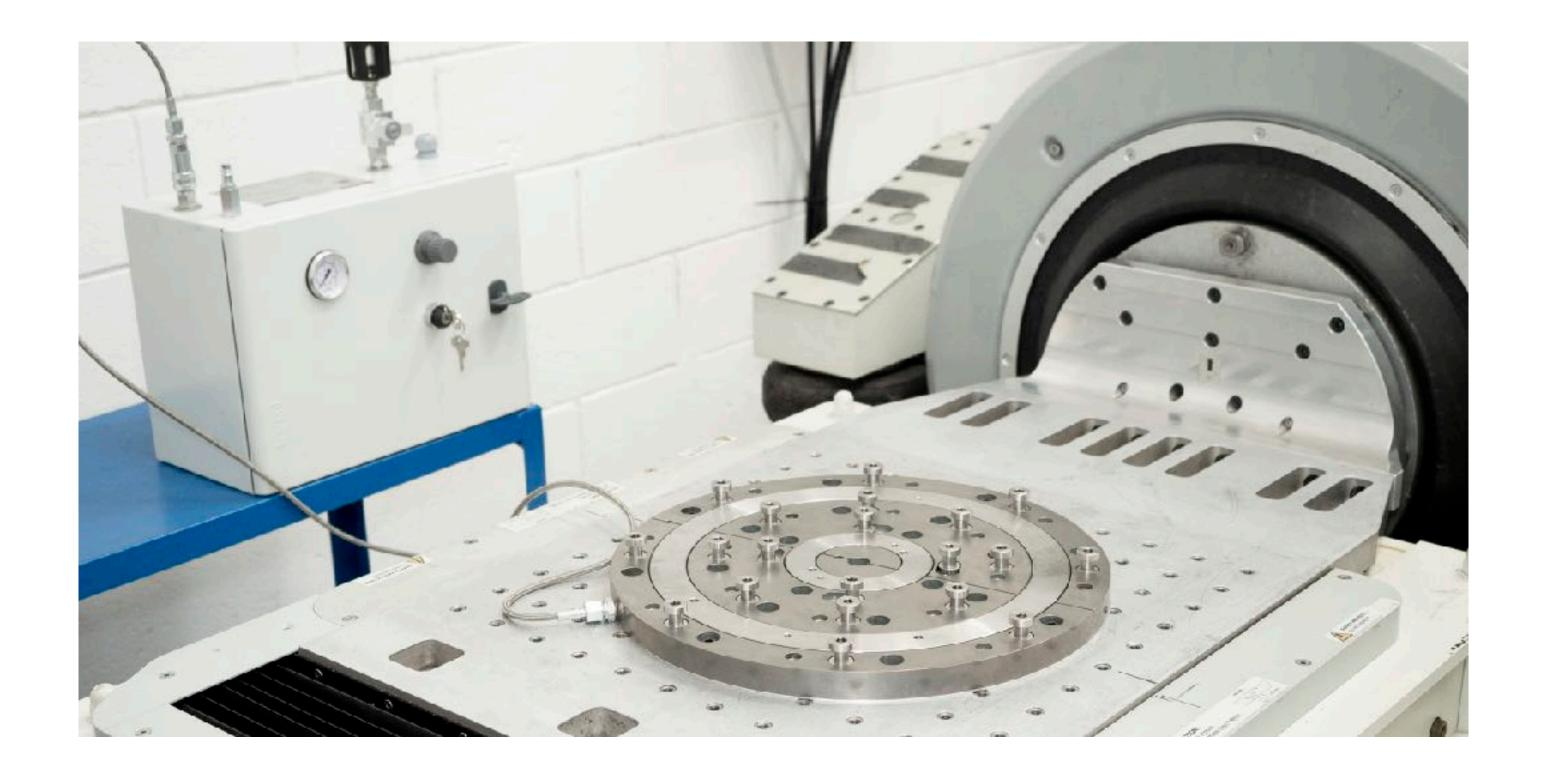
The Instant Clamp can be ordered with standard dimensions for the armature of the most popular shakers or with customizable size and shape.
