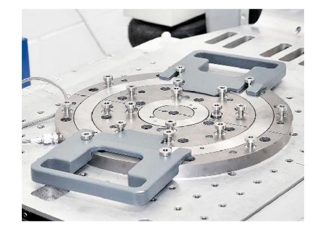
The **tightening is equivalent to the screws** tightened to torque, therefore it's been positively tested both on shaker and slip table, for sine, random and shock tests in a **frequency range up to 2000 Hz**.
