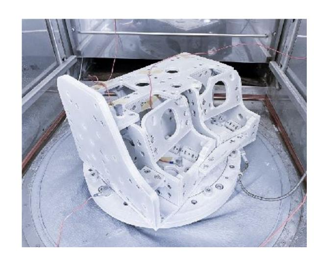
The **Instant Clamp** uses components that allow it to work with a range of temperatures between -40 °C and +160 °C, therefore they are also suitable for combined tests in climatic chambers, an environment in which fixture mounting is usually hard and complex.
