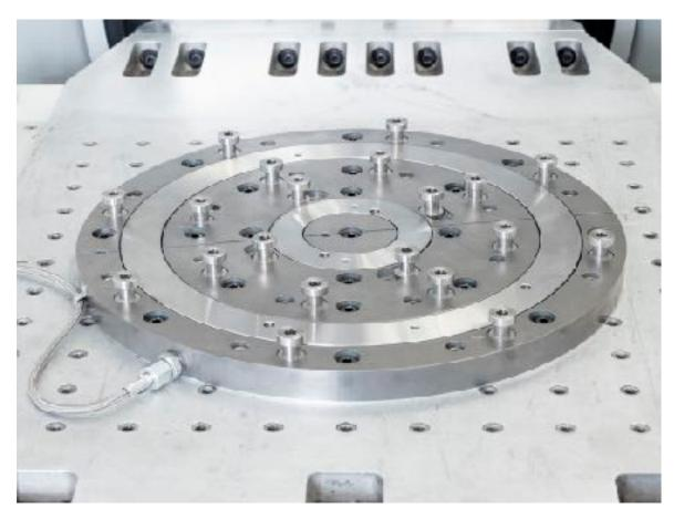
The wedges are accessories designed to facilitate the heavy fixtures manual positioning.
