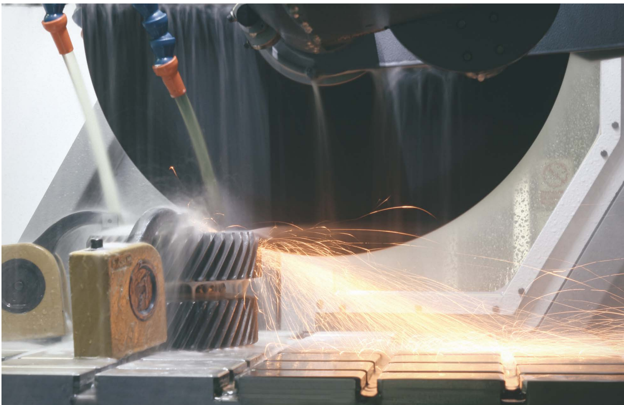
Fast cutting with efficient cooling
