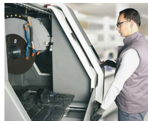
Two Hand Control For Safety Operation
