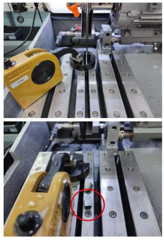
After cutting operation, samples mounted with Diallyphtalat (DAP) polymeric powder in ECOPRESS 102 press.
