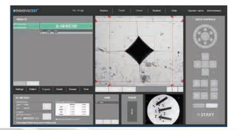
The software supports Kic crack detection under load with customized Kic result reporting. By way of one or both methods, Palmqvist or Median / Radial, fracture toughness is now a repeatable and reproducible test across multiple operators.
