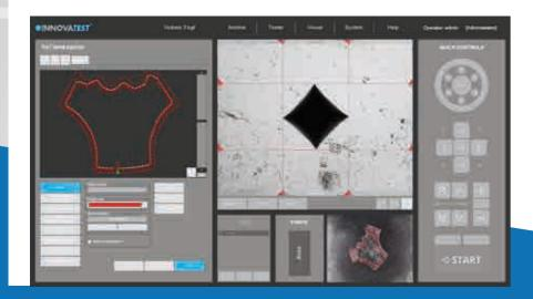
Subsequently, a limitless number of test points can be inserted into the scanned image, or be set at selected distances (offset), relative to the edge. This advanced feature enables the hardness testing procedure to be performed c. An excellent featured combined with 2D or 3D hardness mapping, also known as "plane hardness chart".
