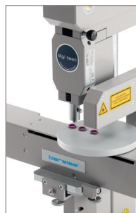
Laser-controlled positioning of O-rings
