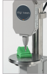
Shore D / C / D0 for finished parts
