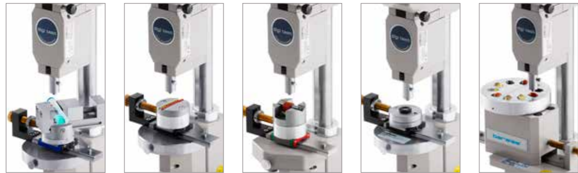
Centering device with vise Centrofix for cables Centrofix for tubes Centrofix customized Rotofix with customized pattern
