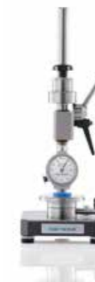
MANUAL TEST STAND, TYPE BS 61 The decision to use a test stand will ensure that the HP is placed at an angle of 90° on the test specimen.
